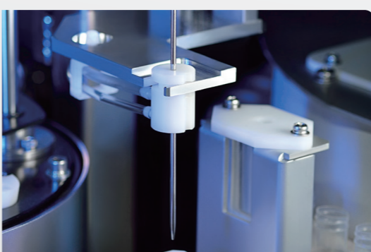
Wiper washing technology Enhance efficiency and minimize carryover
